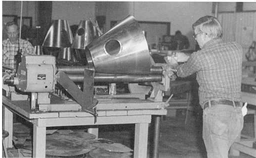
One of many hand forming stations showing the roll forming of a conical shield component. ▶
