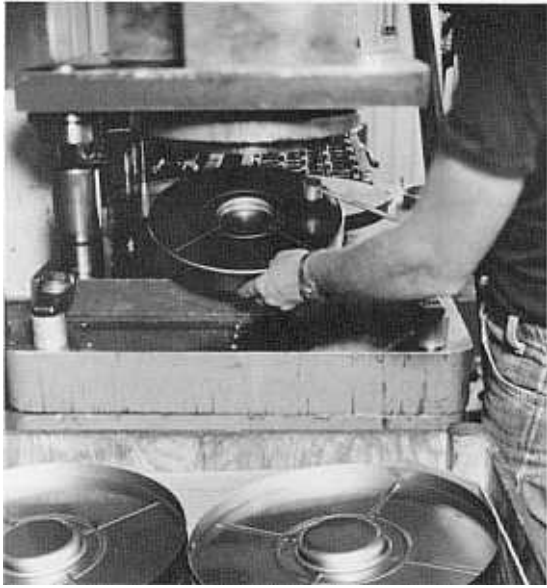
▲ The compound draw and trim die producing tape data protector, P/N TDP 116R15P
