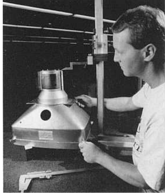
▲ Manual inspection on a 19" color monitor shield by trained individuals with calibrated equipment. Equipment is calibrated to MIL-STD 45662.
