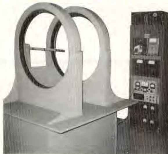
For optimum operation, Ad-Vance Magnetics' in-house Helmholtz testing equipment is built entirely with wood. Even the dowels are wood. There is no metal whatsoever in the frame to distort test results.
