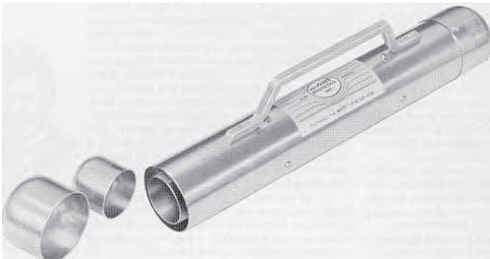
Double-cylinder construction of fabricated alloy provides strength and shape stability for transporting rocks for magnetism studies (left). A large sliding cap fits over the end of each cylinder to minimize any loss in magnetic attenuation from the air gaps.
