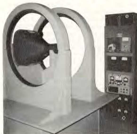
CRT shield testing: The shielding enclosure being tested is entirely contained within the two Helmholtz coils.
