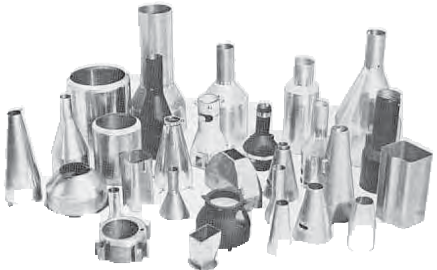
Various CRT shield designs. Wider-spaced, concentric, thin-wall shields are preferred over closely spaced thick shields.
