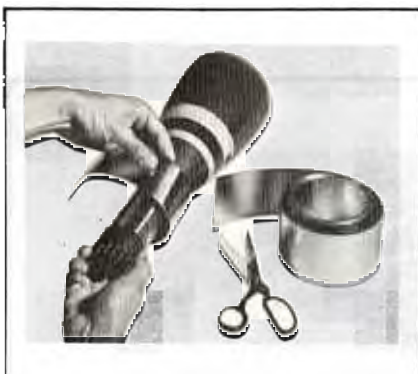
Foil alloy easily cuts with scissors and hand trims to desired outline.
