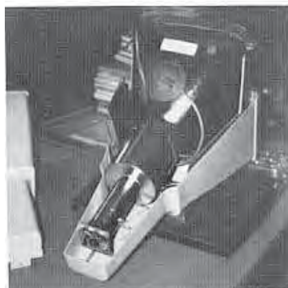
Display unit is designed keeping CRT neck area free of electronic components. CRT with shield (upper); and with shield installed (lower).
