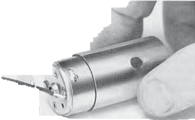
Figure 3: Foil shield wrapped around motor case & foil shielding of cable entry.
