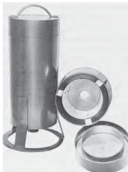
For low-level-field research and for production testing, a magnetic isolation chamber provides an environment in which magnetically-sensitive devices may be observed without interference by external magnetic fields. An operator also can determine the presence of ferromagnetic contaminants in nonmagnetic materials.
