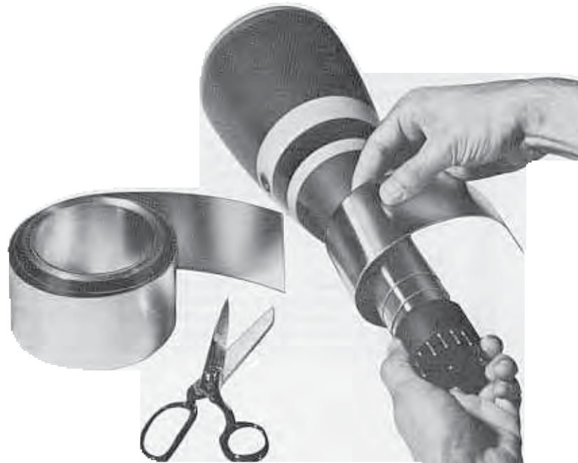
1. A pair of scissors and a roll or two of foil magnetic-alloy material are all you need to fabricate a practical magnetic shield.
